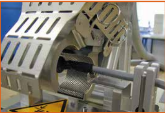
Uniform heat distribution via shrink chambers
