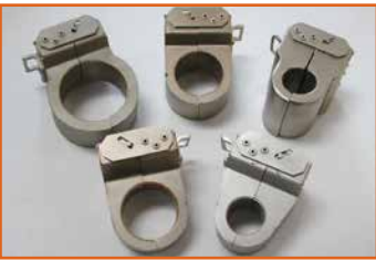
High application variety through various shrink chamber sizes
